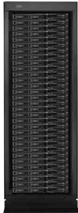
IBM rack populated with System p5 505 and 505Q Express servers
